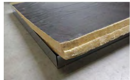
detail 3: different layers of the noise barrier 100 mm non-combustible glass fibre insulation with resistant and water-repellent coating
