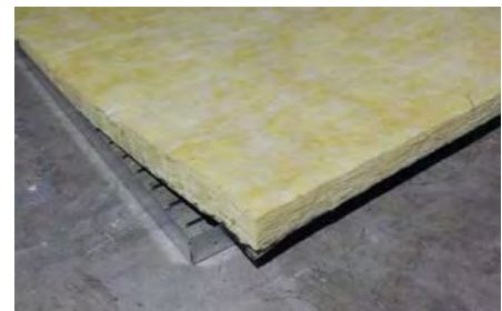
detail 3: different layers of the noise barrier 50mm non-combustible glass fibre insulation with resistant and water-repellent coating
